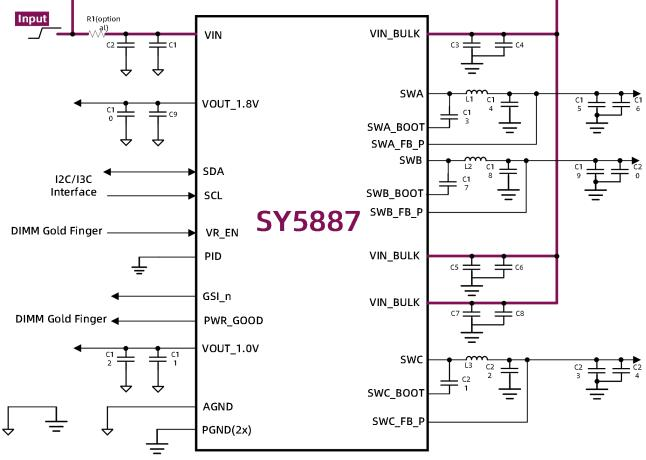
Figure 4- 1. Typical Application Circuit
